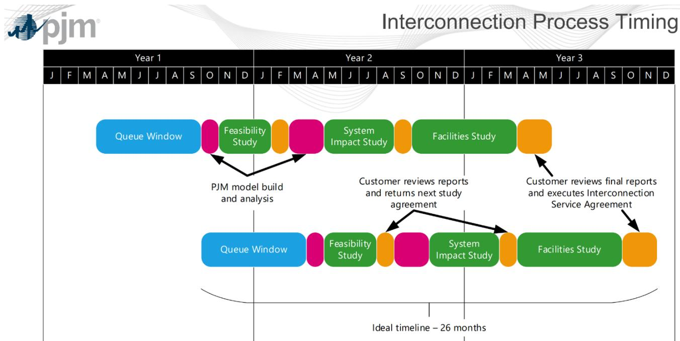
Figure 27: PJM Interconnection Process Diagram and Timeline
