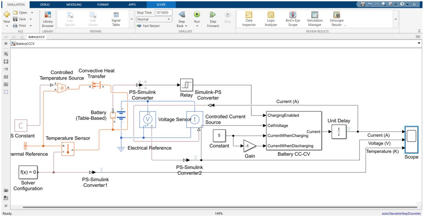
Figure 1 Simulation of CC-CV
