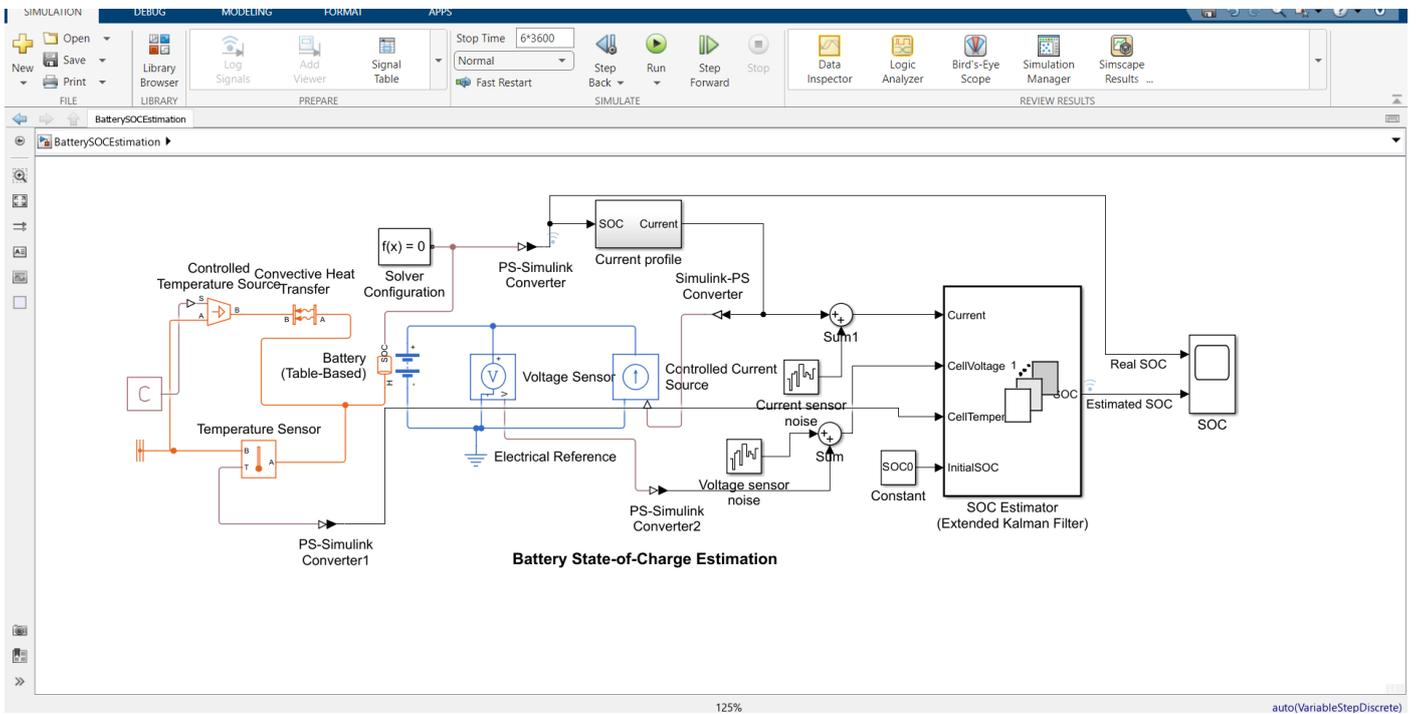
Figure 2 Simulation of SOC Estimation
