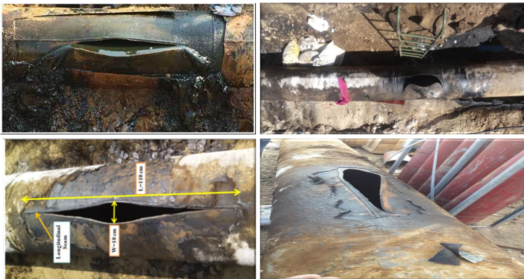
Figure 1.4: AC corrosion damage in District Jamnagar, Gujarat, India (In 2017, burst in 128 days of pipeline commissioning, Source Open)
