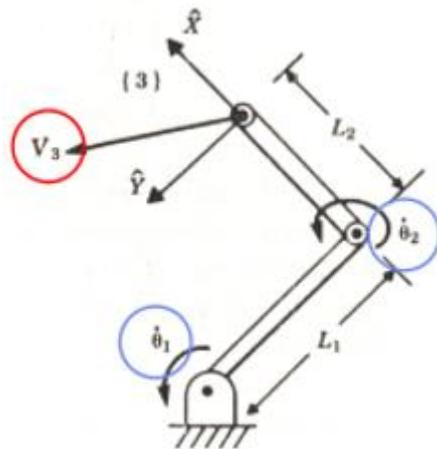
Fig. 3. Schematic diagram of the 2R Manipulator.
