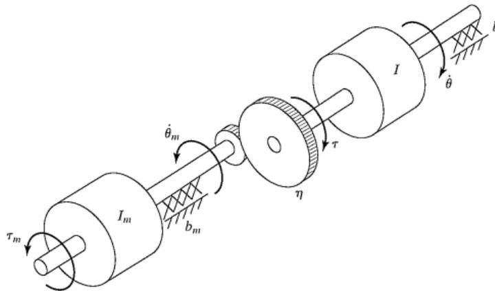
Fig. 6 Single joint rotor system.
