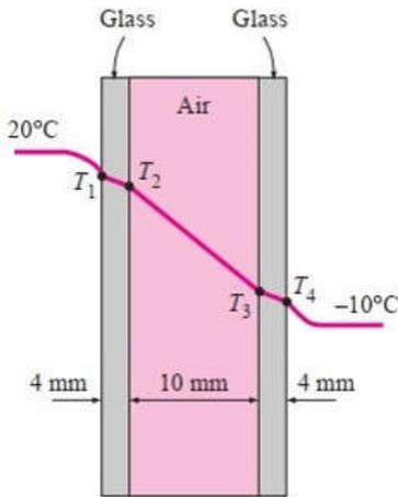
**Fig. 2:** Schematics of the double pane window
