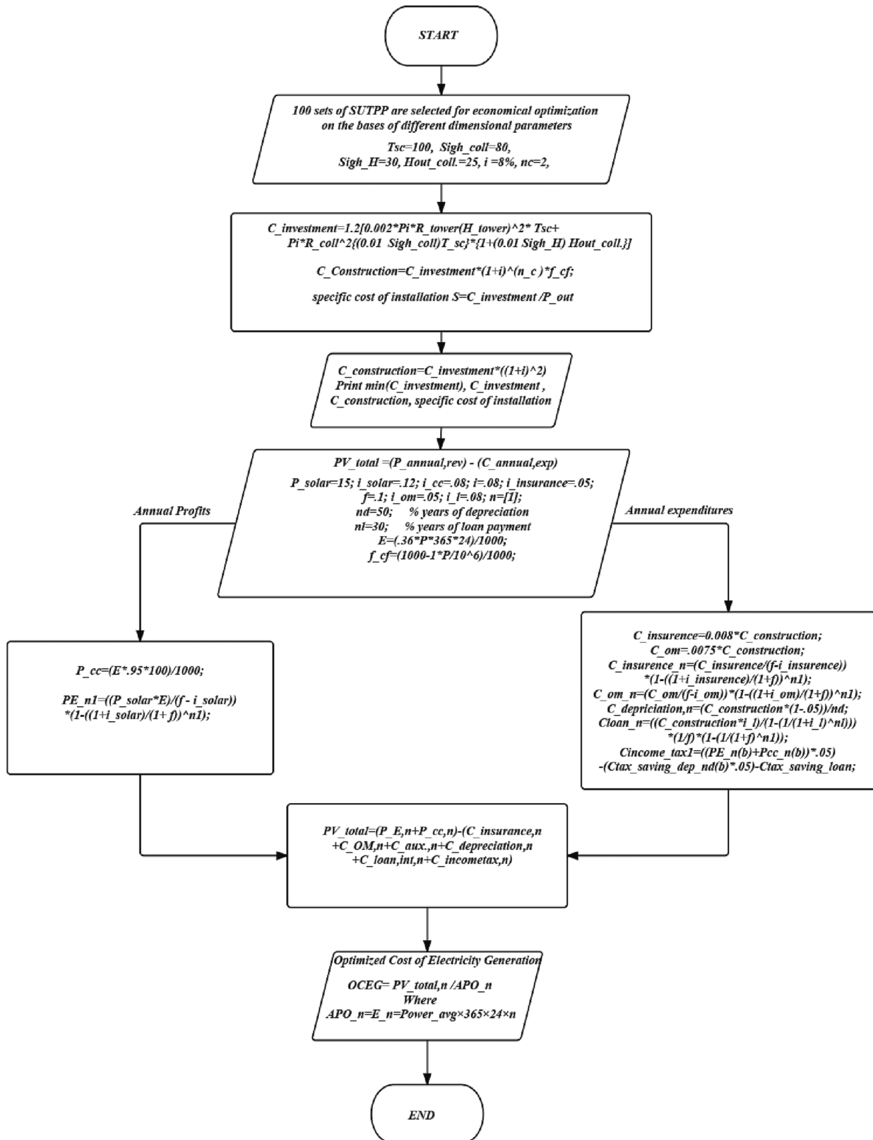
Fig. 1. Flow chart diagram for steps followed to find out the Economic Analysis of SUTPP.
