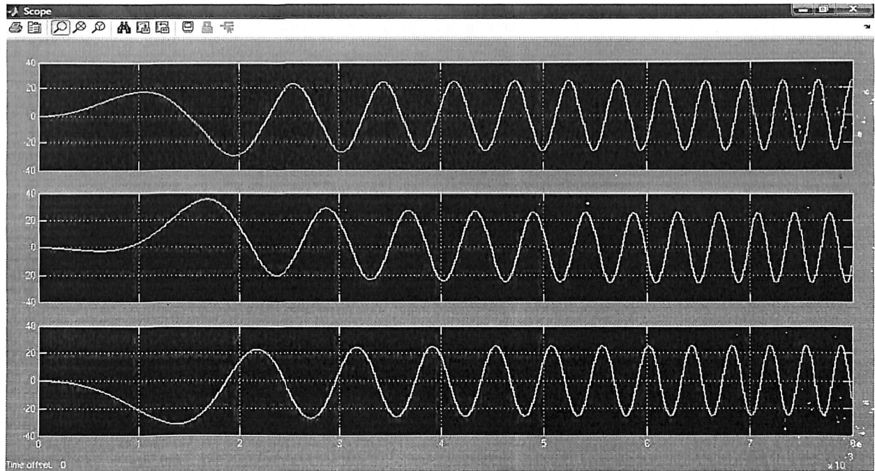
Fig. 4.2 Waveforms of output voltages of permanent magnet generator
