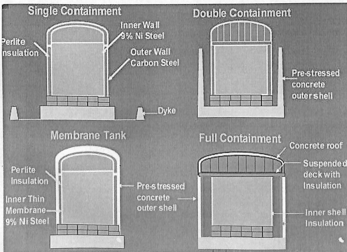
Fig-14 LNG storage tanks
