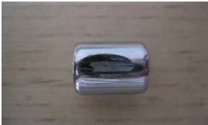
Fig-4.8: Test Specimen (IAS) after Wear Test
