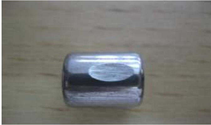
Fig-4.7: Test Specimen (IA) after Wear Test
