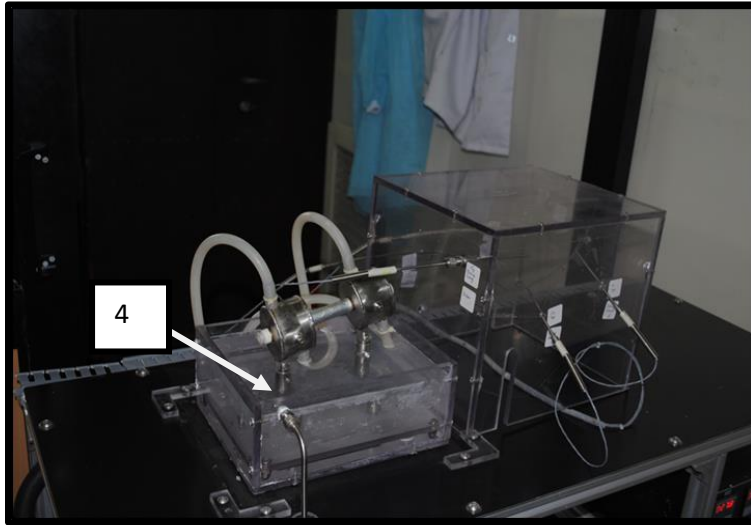
Plate 3: Free circulating water bath adjacent to experimental tube to maintain desired adjacent temperature with the PVC casing.
