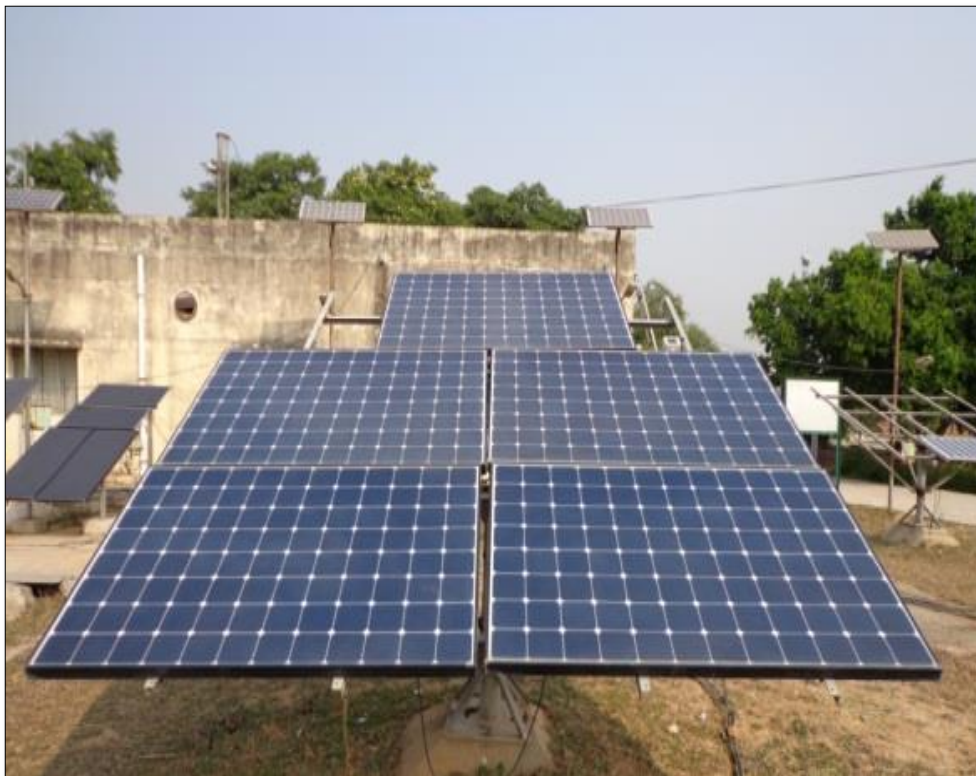
Fig.3.12. A testbed of the SunPower based MAXEON™ technology
