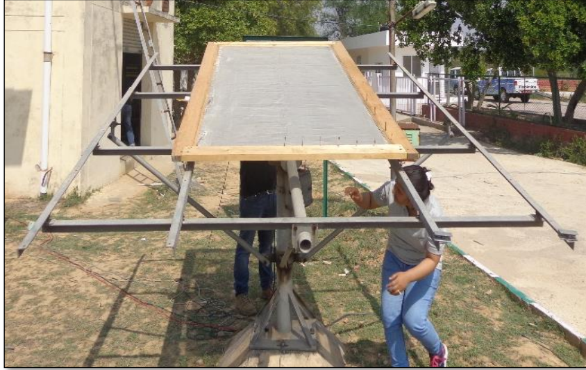
Fig 3.2. Test set-up using mesh for calculation of series resistance of the SPV modules
