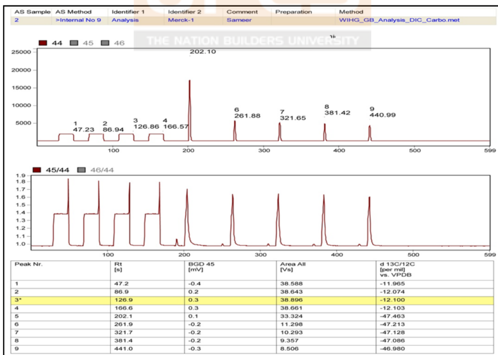
Fig. 3.8: Mass spectrum of Merck (pure, CaCO_3 ) lab standard, measured against reference material of NBS-18 at WIHG lab for use as secondary standard.
