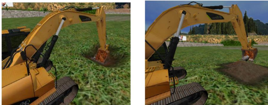
Fig 2.4. Delta3D platform based dynamic excavator simulator
