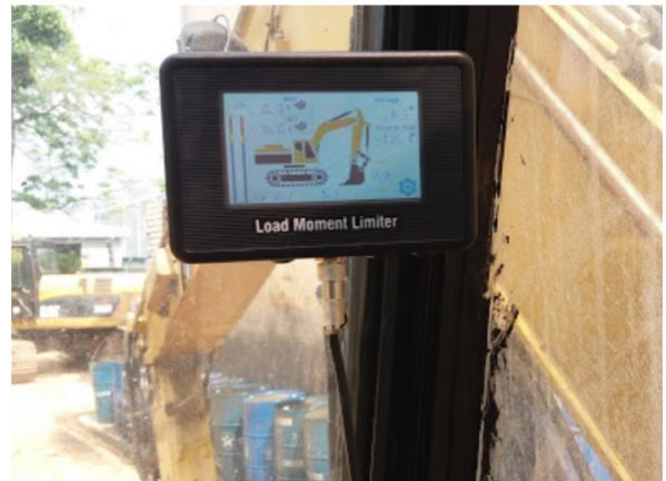
Fig 1.3. Loading chart [11] and visual warning device [12] in excavators
