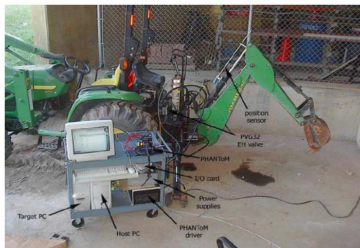
Fig 2.2. Haptic backhoe test-bed [30].
