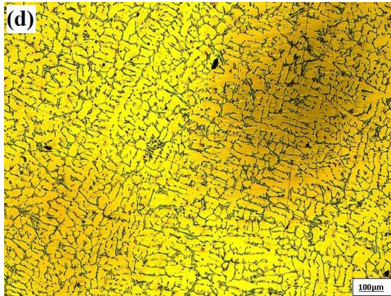
Figure 5.2 Microstructure of AS alloy & its composites (a) Al-Si (b) ASV1 (c) ASV3 (d) ASV5
