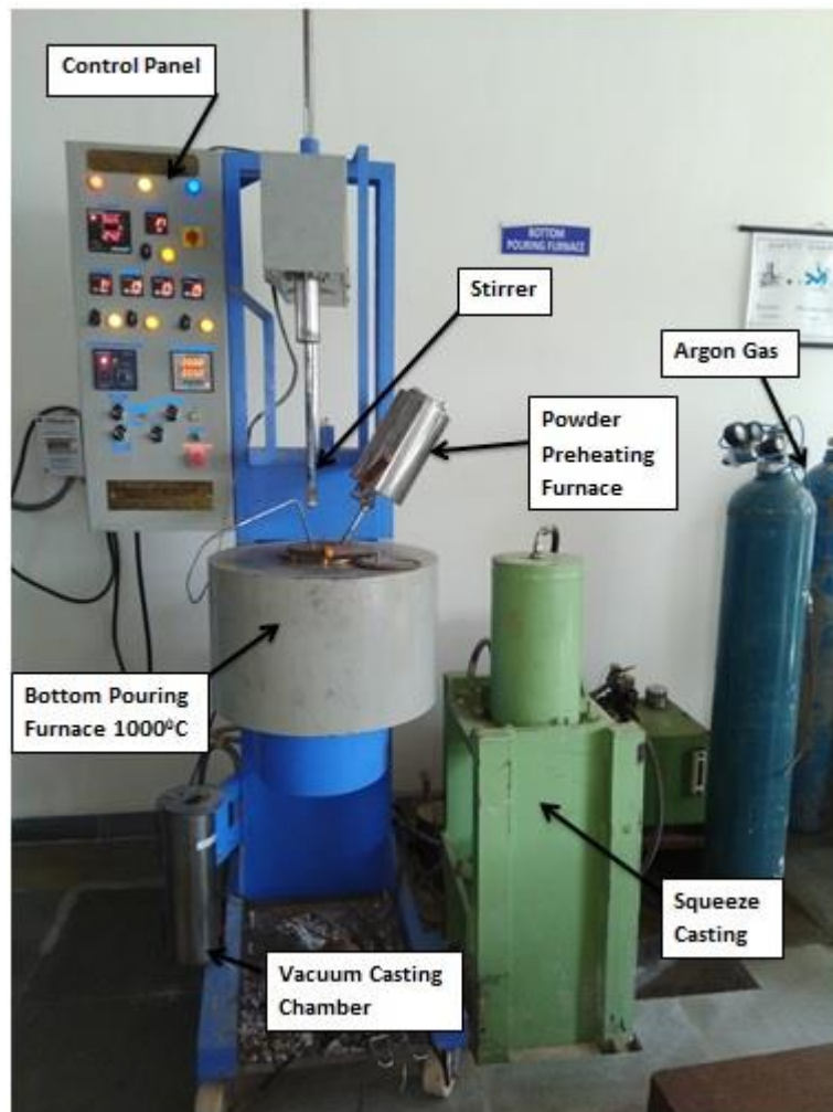
Figure 3.2 Bottom Pouring Stir Casting furnace
