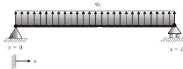
Find the appropriate approximation for deformation  $v(x)$  using the Principle of Stationary Total Potential (PSTP).
