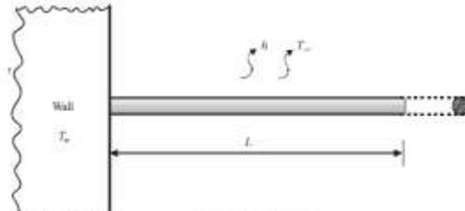
$$k \frac{d^2T}{dx^2} = \frac{Ph}{A_c}(T - T_\infty); \quad T(0) = T_w = 300^\circ C, \quad \frac{dT}{dx(L)} = 0$$
