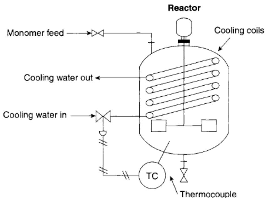
**Figure 10-8** An exothermic reaction controlled by cooling water.
