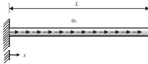
Q 9 Consider a 1 mm diameter, 50 mm long aluminum pin fin as shown in the fig. that is used to enhance the heat transfer from a surface wall maintained at 300°C. The governing differential equation and the boundary conditions are given by,
