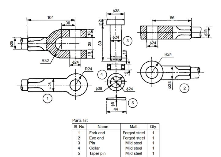
Figure 2 : Details of a Knuckle Joint
