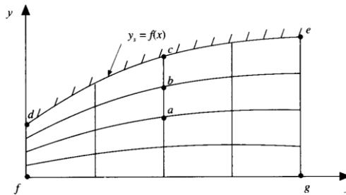
Fig. 1 Section of a divergent duct in the physical plane
