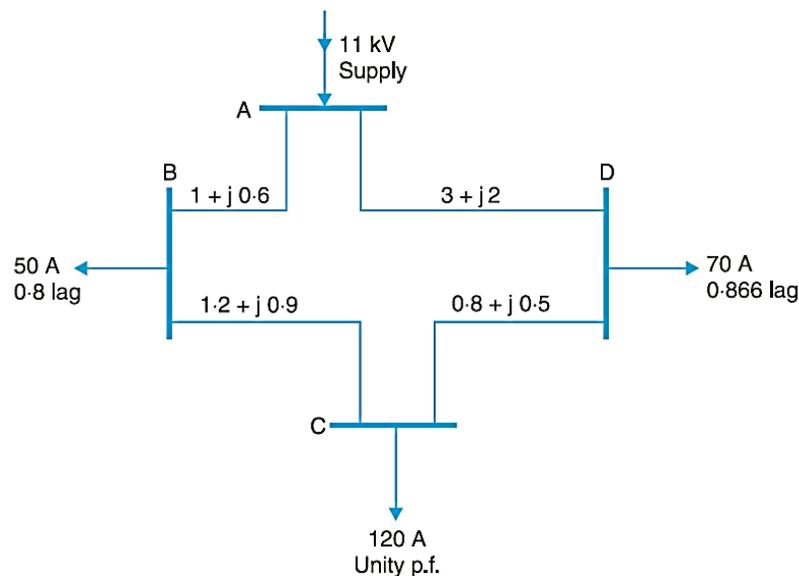
Q.No.10 A fertilizer industry is connected with following loads:
