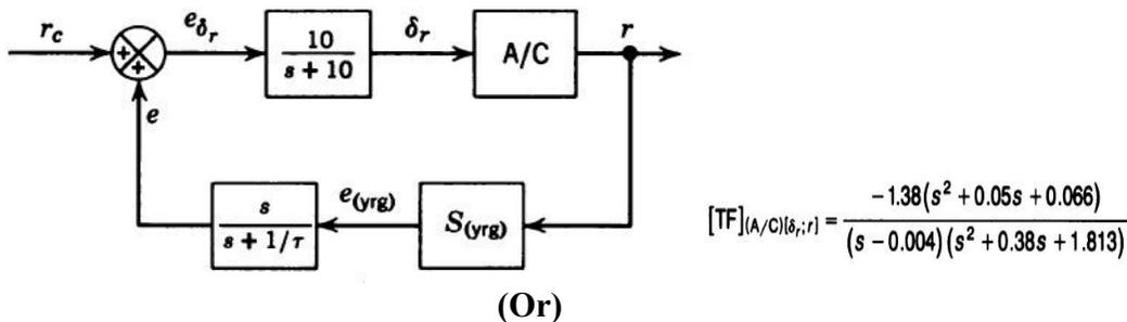
Q 10 Write the MATLAB Programming for lateral autopilot from Figure 3. Time constant 5 sec and Find the closed loop transfer function.
