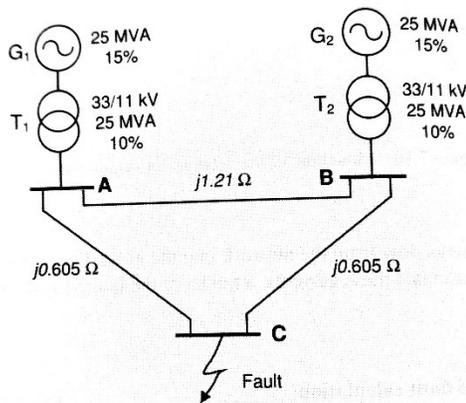
For the power system shown in above fig, draw the network diagram giving all reactances on 100 MVA base. Calculate the fault current in pu and in amperes for a three phase short circuit fault at C. all pre
