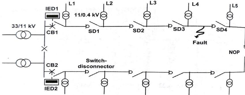
The figure represents a typical 11 kV distribution network section. IED1 & IED2 consists an over current protection element. The fault occurred in between SD3 and SD4. Restore the supply in less span time is the main objective. Considering the data given,
