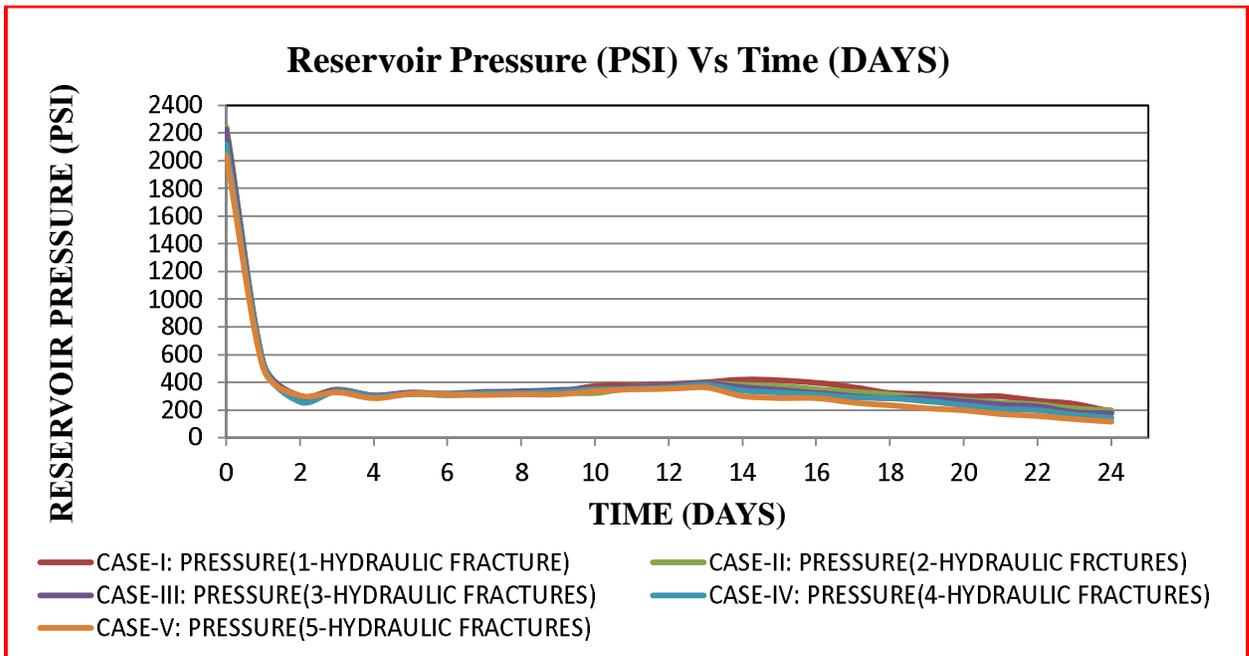
Figure 8.8: The pressure variations in reservoir versus time at different fracture stages.
