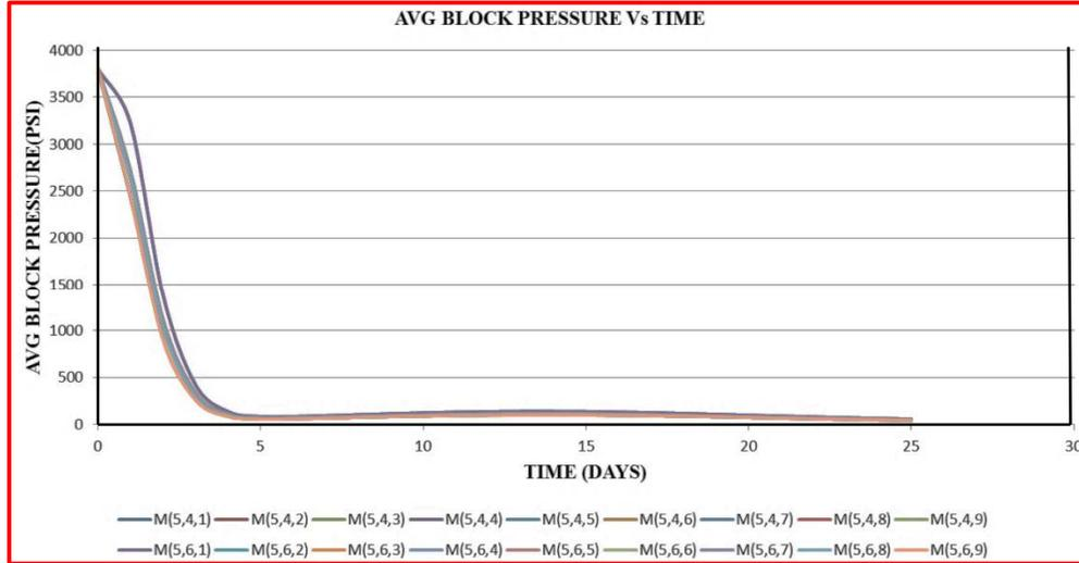
Figure 5.2: Individual matrix block pressure variation with time.
