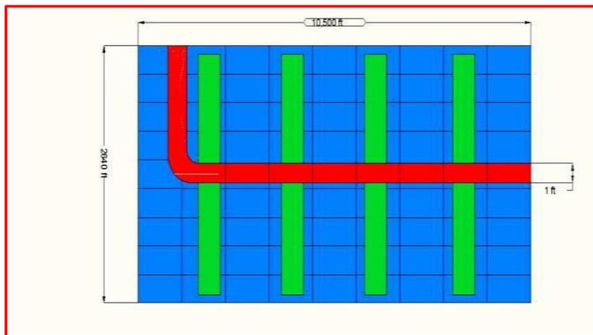
Figure 5.4: Schematic representation of shale reservoir with horizontal wellbore and four Hydraulic fractures.
