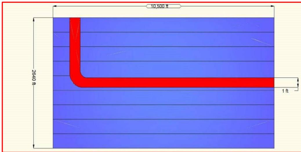
*Figure 5.1: Shale reservoir with horizontal wellbore and no hydraulic fractures.*
