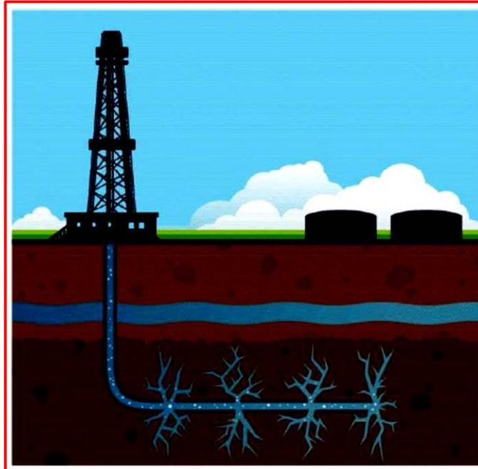
Figure 1.7: Horizontal drilling and multi-stage hydraulic fracturing (Web Page)
