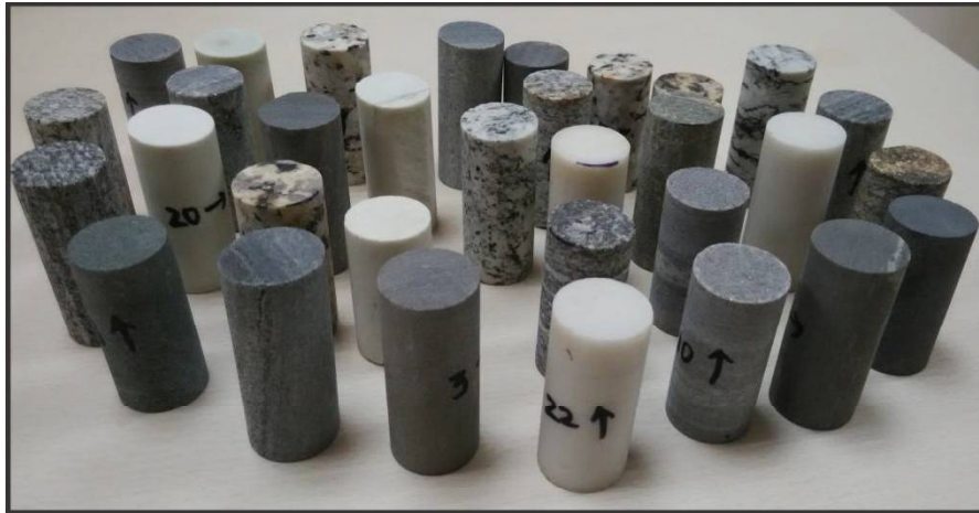
Figure 5.13 Photograph showing the cylindrical cores samples.
