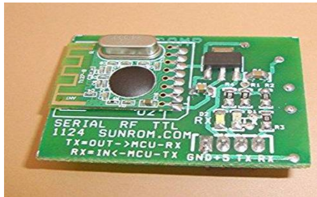
Fig.3.4 RF modem (model no.-1124 from Sunrom)
