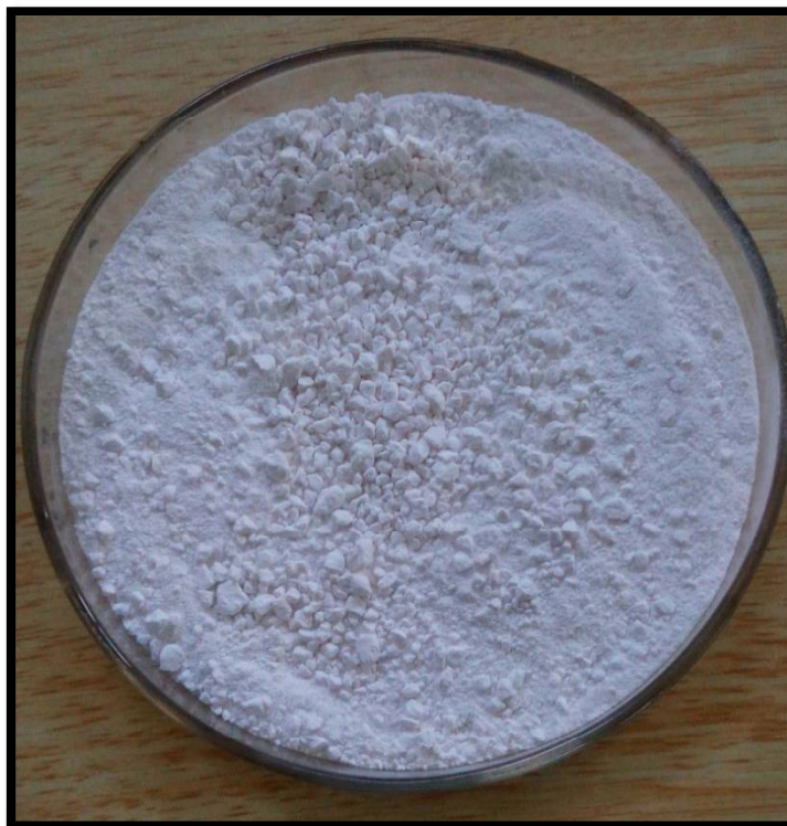
Figure 3.17 Zirconia powder after calcination
