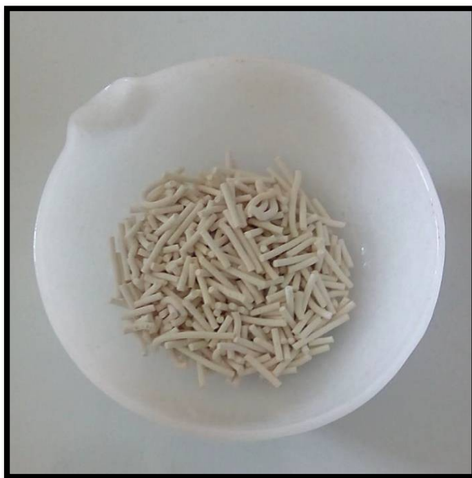
Figure 3.8 Sulphated Zirconia after impregnation of TPA
