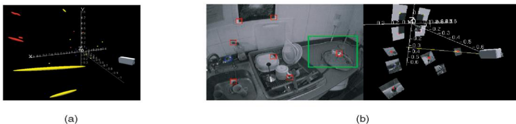
Fig. 2.5: (a) A snap shot of probabilistic 3D Map showing camera position estimate and feature position uncertainly ellipsoids (b) visually salient feature detected.
