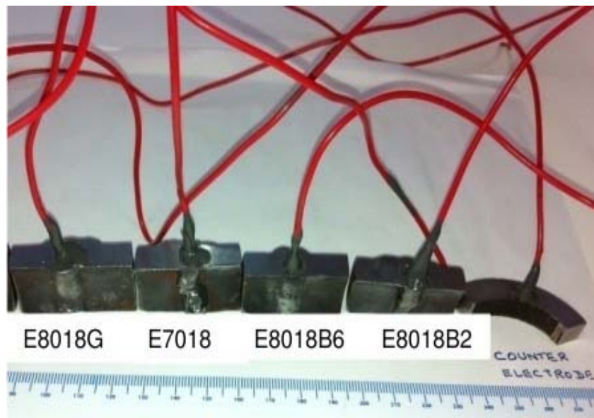
Figure 3.6: Weld Samples Prepared for Corrosion Testing
