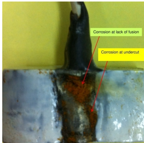
Figure 4.14: Corrosion Tested Weld (E7018) with Lack of Root Fusion and Undercut
