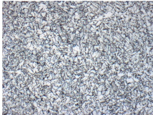
Figure 4.3e: E8018B6 Weld Metal at 200X for 6-9 'O' clock position
