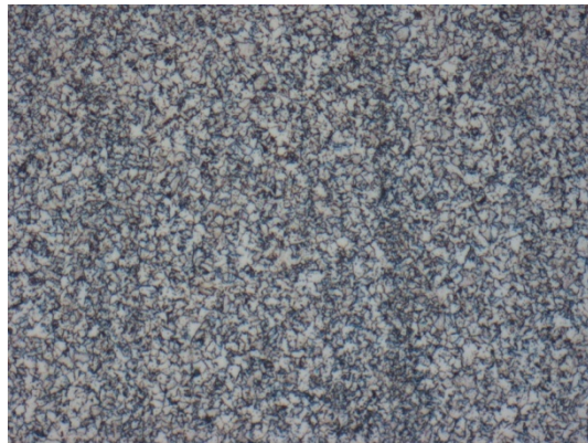
Figure 4.3h: E8018B2 HAZ at 200X for 6-9 'O' clock position
