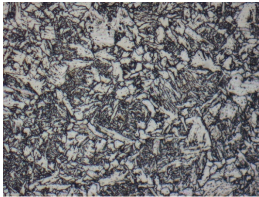
Figure 4.3a: E8018G Weld Metal at 200X for 6-9 'O' clock position
