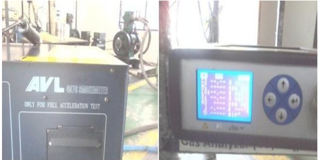
Fig.3.7: Smoke meter and Exhaust gas analyzer
