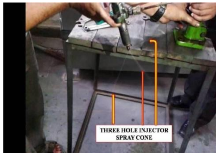
Fig. 3.5: Three hole injector and the spray cone
