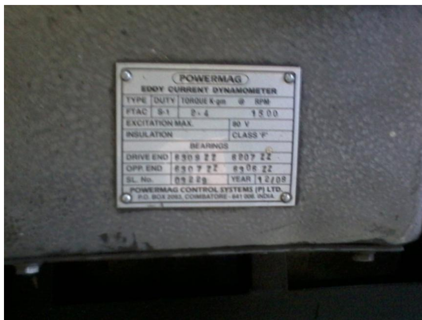
Fig. 3.6: The eddy current type Dynamometer
